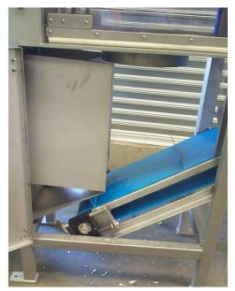
The Segmenter is a self-supporting smooth, quite running design constructed from stainless steel and food grade plastic components with a glass beaded finish.
