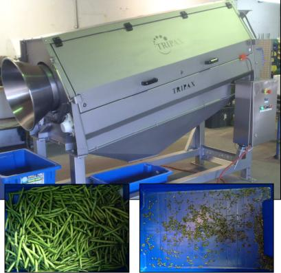
housing trunnion wheels at either end. Then you have a drive end which is powered by an SEW geared drive shaft mounted, motor transferring transmission through a series of timing pulleys and belt, whilst the idler end is simply a driven motion via the drive of the drum rotation.
