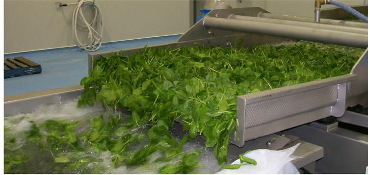
**Function:** To accept product from washer, Conveyor, bin tipper or Crate to dewater and separate running or residual water from the product as well as remove unwanted solids or bugs within the product mix, as well as performing an even continuous feed of product in the production line.
