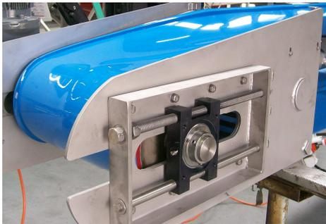
The conveyor comes with optional features like: Top hood and under belt covers, discharge guides, chutes and scrapers for removing sticky products from the belt. This design is fully open and extremely easy to clean down and access the underside of the belt and its forward and return guides, which are all static and don't require any future maintenance apart from replacement when worn.
