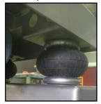
The air bags are controlled via an inflation manifold with a gauge to enable the user to adjust the hardness of the isolation that effects the settling action, sometimes softer for some products and harder for others. The settling table
